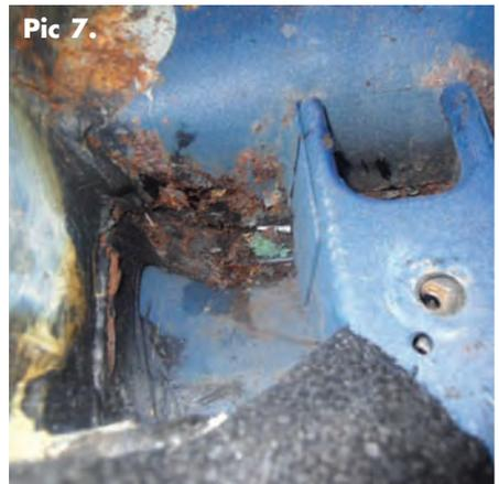
Picture 7. shows the point where the rear trailing arms attach. This is pictured from inside and I can assure you it looks worse underneath.
