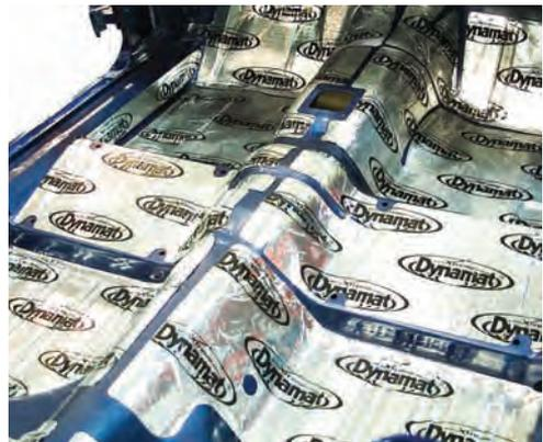
**A:** We recommend applying Dynamat to any surface you can easily reach. In general, we recommend treating your vehicle in the following order: Doors, Boot, Rear Deck, Floors, Roof, Bonnet, then Bumpers.
