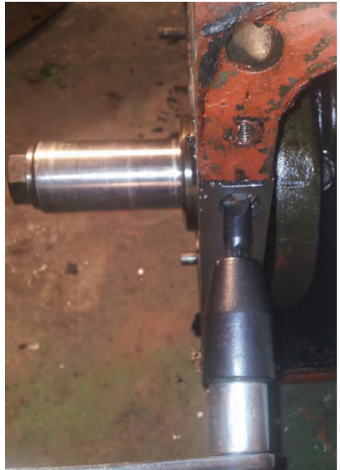
Photo 3: Front sealing block being torqued up
