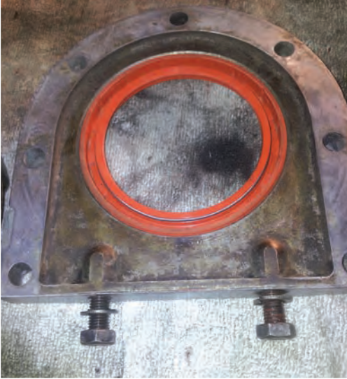
Picture 2: Rear seal fitted flush with its housing
