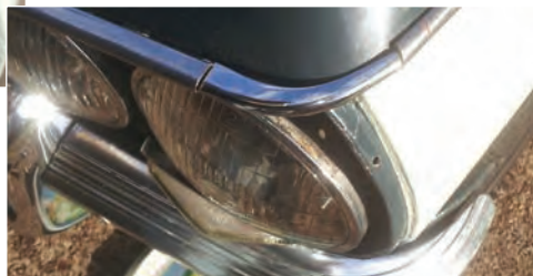
Picture 8: The new moulding fixed in place
