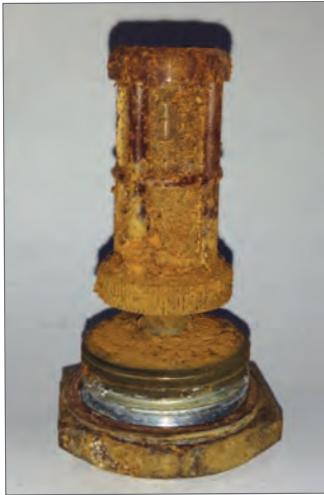
Picture 2: Blocked Estate tank outlet assembly
