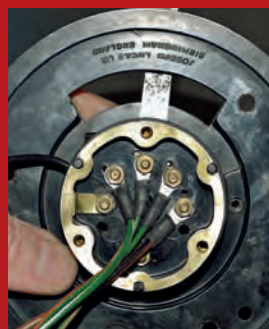
TR2/3 LUCAS HORN/INDICATOR CONTROL Huge tech guide to repairing this costly unit.
