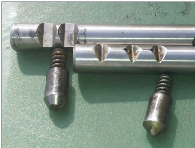
Photo 1: Reverse selector rod and plunger (left and upper) and 1st/2nd rod and plunger
