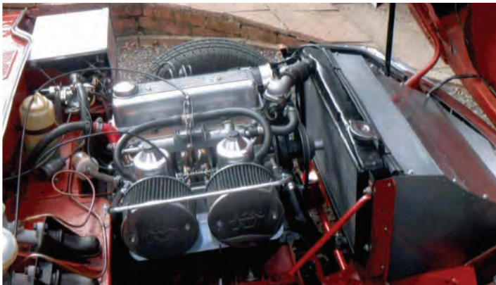
General view of engine bay (note air receiver in front of oversized radiator, that also has a lower air scoop)
