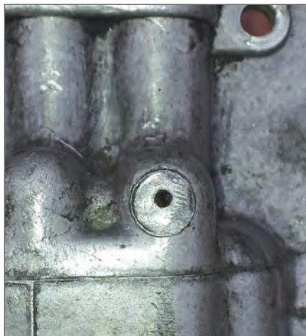
Photo 5: Oil and access hole above the reverse plunger
