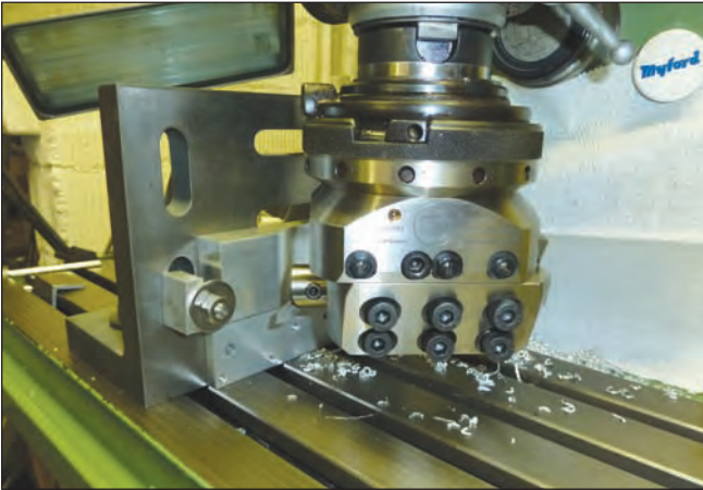
Machining of the mounting block for the servo in the 1500 Spitfire.
