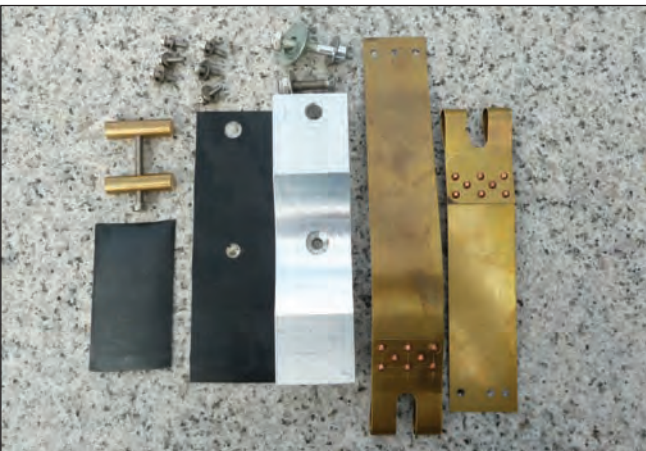
View of all the parts for mounting the servo in the 1500 Spitfire.
