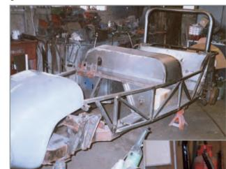
The body was clad in 1.5mm half hard aluminium, using a series of cardboard templates to cut the correct shapes from the flat sheets of aluminium. The rear panel, having to be bent around compound curves, was heated up to soften it sufficiently. The bonnet was again made using a cardboard template with the curved edges being formed using a large welding bottle. This process took five days over three weekends, and this was using an
