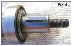
method which involves removing the front pulley and woodruff key (pic 4), then gently tapping the shaft out through the rear of the housing. This only becomes possible once the bearing-retaining circlip has broken and the pieces fallen out of the housing. This was what had caused me to retire the unit back in 2008 - now I know where the bits actually came
