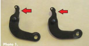
Photo 1 shows the arms from Suzie's Mk III Spitfire and wear can clearly be seen where the arm abuts the brake shoe. Photo 2 shows the arms following a bead of weld being added to fill in the worn section and then filed down to rebuild them to their original shape. When refitted I had to significantly adjust the handbrake cable which showed the effect of the wear. An hour after doing this we had an
