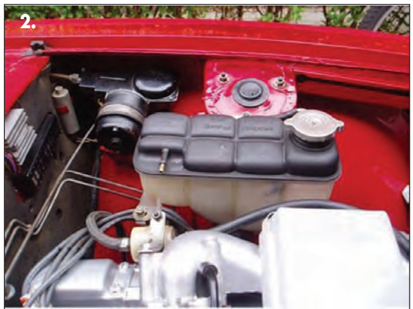
Picture 2. Tank in trial fitted position on the nearside turret.
