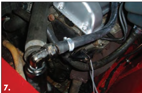
Picture 7. Plumbing connection into the top of the radiator
