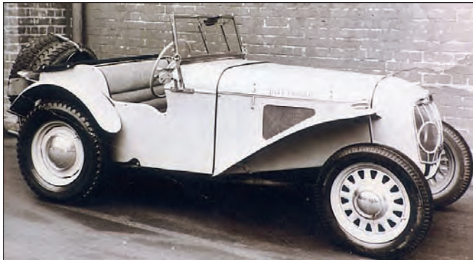
Buttercup trials car with Standard 8 Chassis and fitted with a Vanguard Engine
