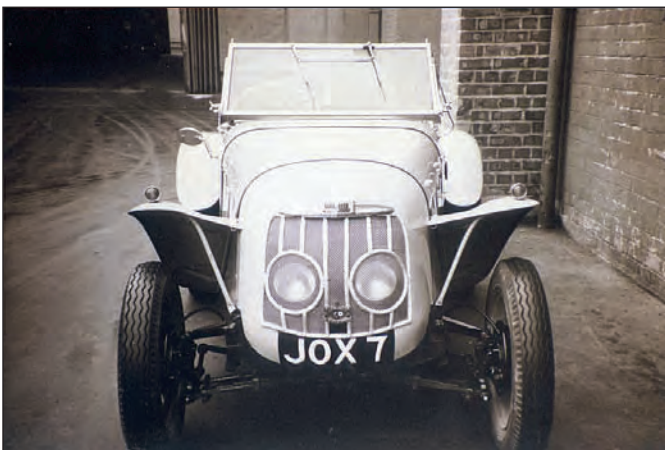
Buttercup trials car with Transverse Leaf Spring Front Suspension
