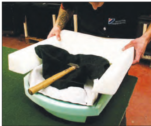
Glue edge contour foam to base
