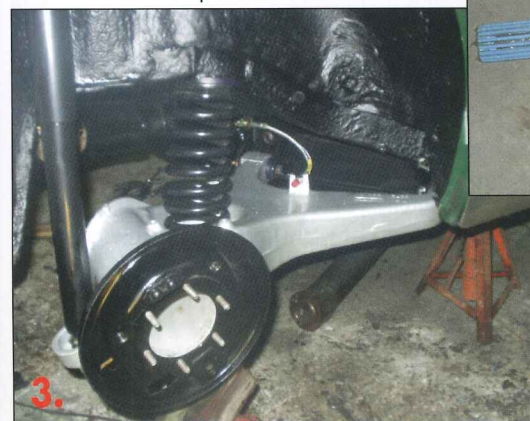
studs on the alloy trailing arm Photo 2 shows the back plate and brake wheel
