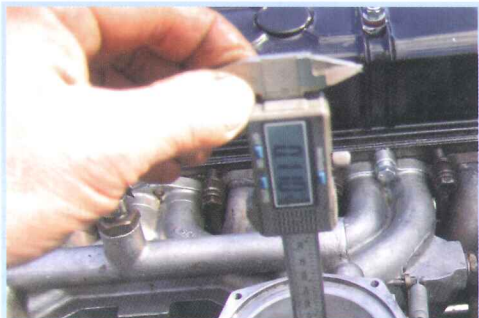
Measuring jet heights prior to final adjustments
