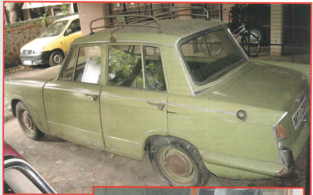
fuel tank opening on the rear wing closed, the tank being accessible only from the boot. Many car owners (especially of Heralds) in India have done this modification, owing to
