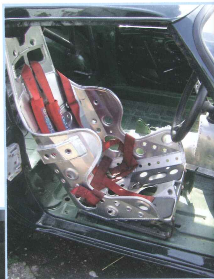
Photo 2 Welded to Measure – the bespoke Nascar seat
