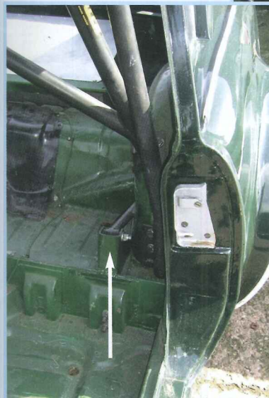
Photo 5 The anti-tramp additional rear suspension arm (inboard of the rally cage)
