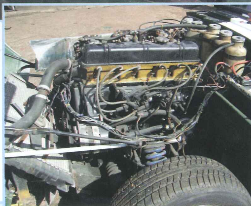
Photo 7 The Cosworth mapped Ignition system
