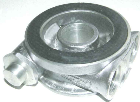
Fig. 3. Sandwich Plate with built in thermostat
