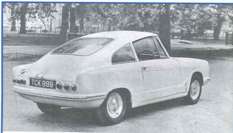
As the bumper strips contact the glass fibre body, minor accidents could do major damage; but they extend sufficiently to protect the lamps at front and rear. Amber turn indicators are on the outside, combined brake and tail lamp in the centre of each group, and the inner ones are reflector
