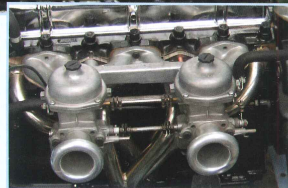
Stromberg carburettors (shown) can be changed for SU 1 1/2"
