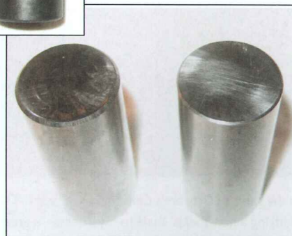
This picture shows the hand ground radius (left) to the C & C machined OE spec (right)
