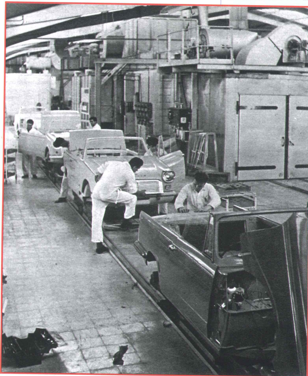
The assembly line with the spray booth and drying ovens in the background.
