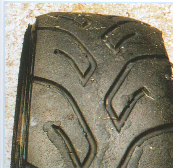
Tyre Shredding at cadwell - I was lucky it cut into the tread and not the sidewall!
