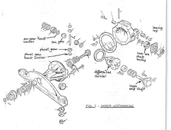
The strengthening of the internals of the diff. affects the inner axle shaft, planet and sum gears and differential carrier (see Fig.1). The inner axle shafts of the 13/60 have a bearing journal diameter of 25.011 - 25.024 mm as opposed to 22.215 - 22.225 On early 1200's. There are also 20 external serrations for
