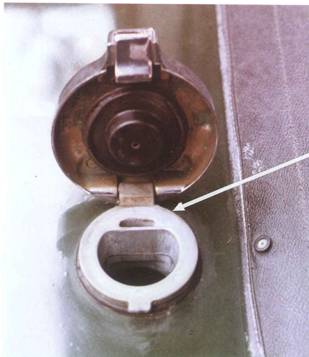
Fig 3. Filler Neck Seal. These seals are particularly prone to leaking
