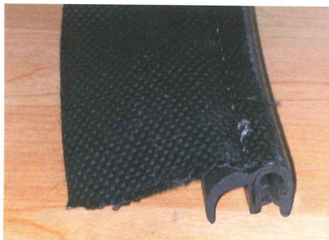
Stitched from above, between lip and seal body
