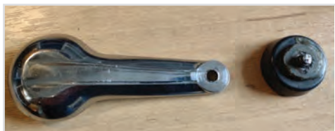
Broken handle, the knob broke off.
