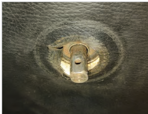
Window Winder shaft with hole for securing pin
