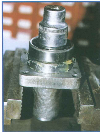
Fig. 9 Using the old bearing and a socket as shown, drive the new roller bearing squarely into the housing.
