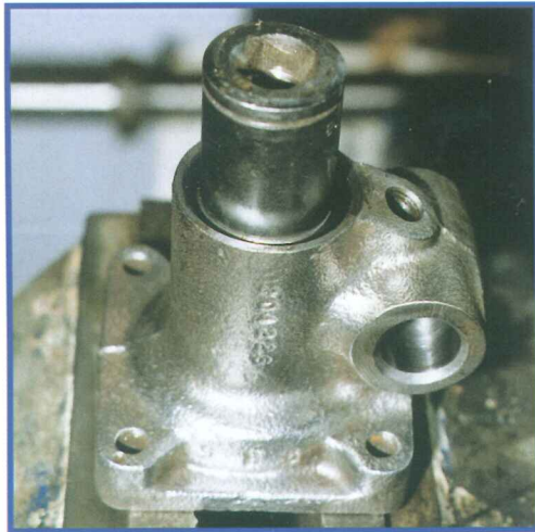
Fig. 8 Using a large socket, tap in the new needle bearing, lettered end trailing, followed by the new oil seal, with the lips and 'spring retainers' trailing, i.e. facing outwards.
