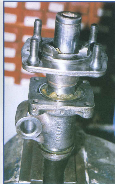
Fig. 11 Refit the flinger/stone guard, followed by the bearing housing. The question is how far along the shaft do you push/tap the housing? The method I use is to use the hub and socket as shown to drive the housing down the halfshaft until the hub reaches the halfshaft taper. Make sure you grease the taper, otherwise you won't be able to remove the hub again!
