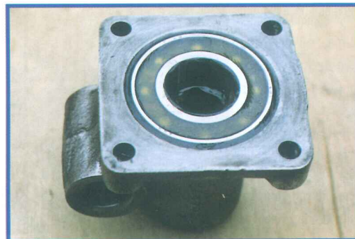
Fig. 9 Using the old bearing and a socket as shown, drive the new roller bearing squarely into the housing.
