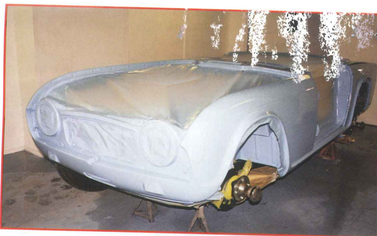
Body Back on new chassis wings and doors being fitted and aligned before last colour coat
