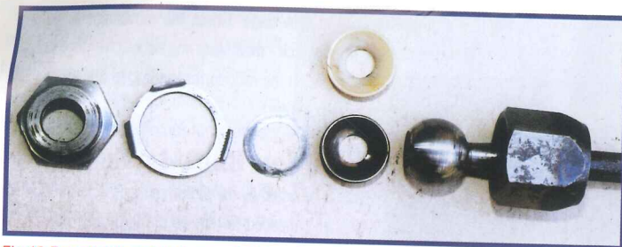
Fig 10 From left to right: sleeve nut, tab washer, shim, cup (steel or plastic), track rod, cup nut
