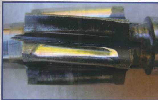
Fig 7. Excessive wear in the pinion.
