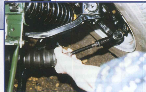
Fig 3 Check for wear in the bush in the end of the rack tube.
