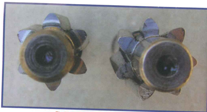
Fig 5. 4-cylinder cars use 6 tooth pinions, 6-cylinder cars have 7 tooth pinions.
