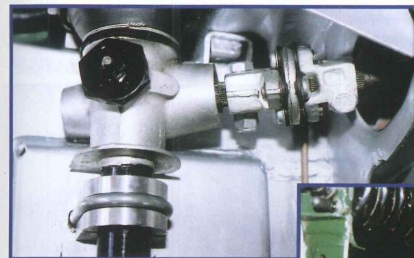
Fig 1 Solid rack mounts and steering coupling. On early cars, ensure that there is an earth lead between the 2 pinch bolts and another from the grease nipple to the chassis, otherwise the horn won't work
