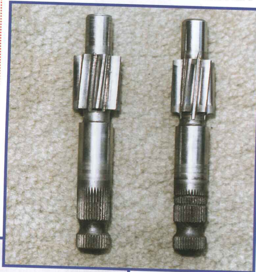
Fig 6. Grooves in the end of the pinion denote its intended use on a 6-cylinder car.
