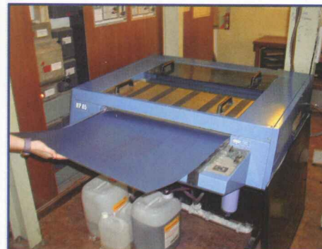
Each plate is then put through a chemical bath to process the plate ready for printing
