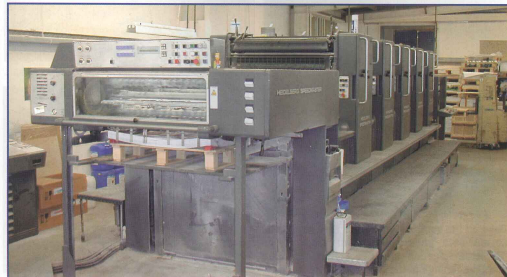
Each plate is placed onto the colour printing press ( one colour per cylinder) ready to print (Above)
