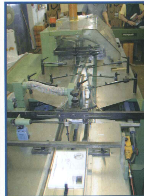
Each magazine has its unique address label attached and is then sealed inside the Polythene carrier which is cut and heat sealed.
