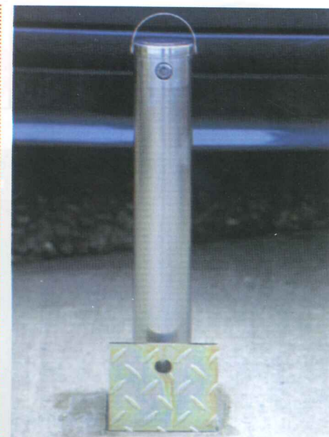
The Driveguard post extends telescopically from its oil bath and drops clear out of the way when not in use. A similar post is available for trailers too.
