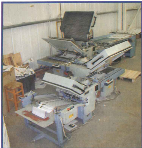
Once the flat sheets are done they are then folded into the finished sections.
