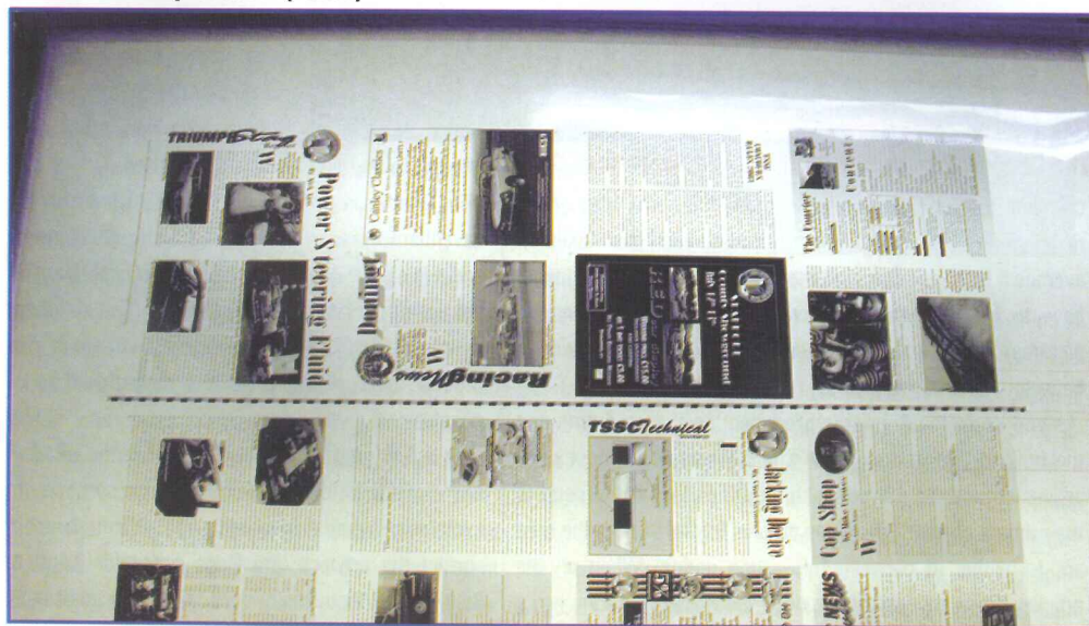
The films are then checked for quality, 4 separate films made ready for plate making. (Above)
