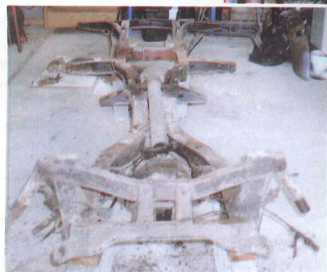
Chassis stripped and ready for blasting.
