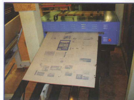
Each plate then matches the original film, as you can see each plate has 16 Courier pages on it, or in print terms '16 to view'
