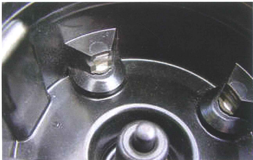
Fig 1. Grooves worn in the terminal posts of distributor cap.
