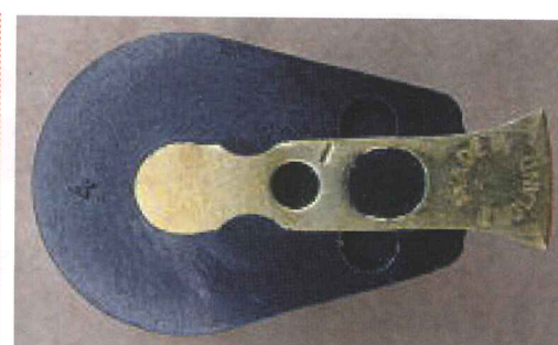
Fig 7. The alternative CI design which mimics the original Lucas design.
