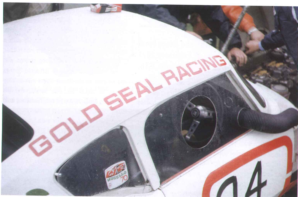
All GT6's Get Hot inside! Note: large Drivers air duct through window
