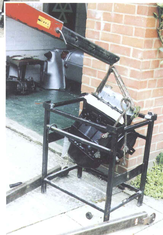
Fig 3. Lifting the engine out of the Transport Cradle. With the engine hoist this is quite easy.
