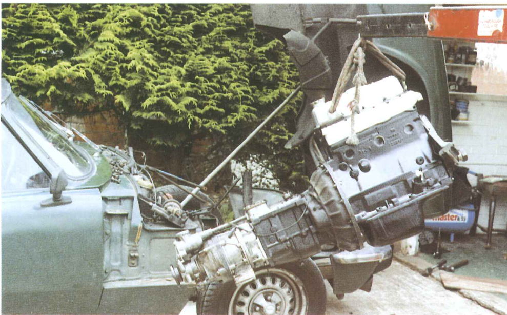
Fig 5. The engine/gearbox ready to go back in. I use a tubular exhaust manifold and so this and the Inlet manifolds have to be refitted in the car. Note the angle of engine on the hoist - this is quite important for manoeuvring into place. Note the Broom handle propping the bonnet open as wide as possible
