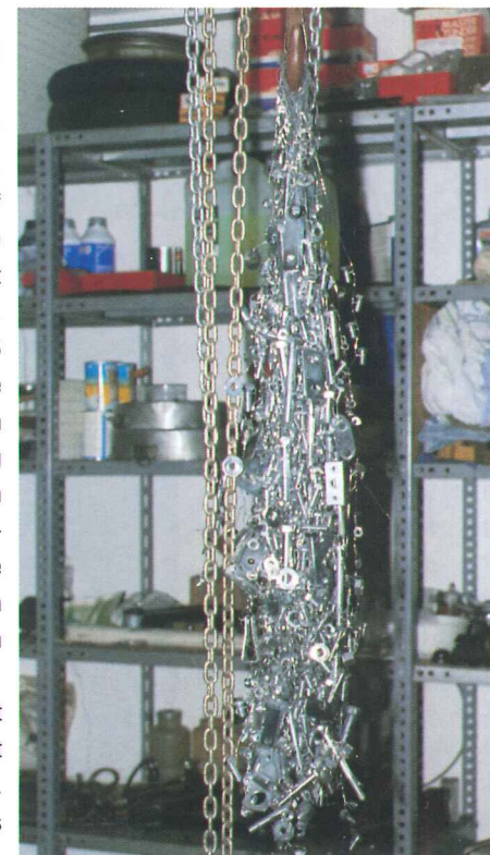
Fig 2. All the nuts and bolts etc. after being galvanised
