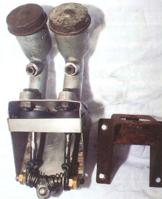
9. Adjustable Bias Twin Master Cylinder for braking system
