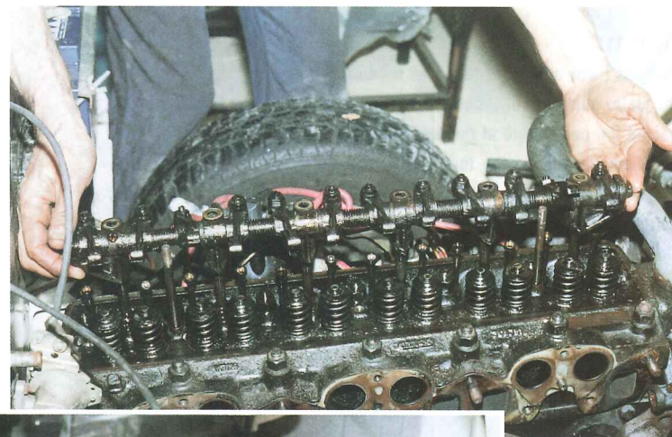
Figure 8. After removing the rocker cover, gradually release the rocker pedestal nuts and remove the rocker gear.
