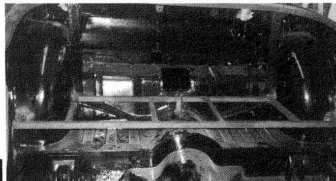
Front panel to the security locker system in place; note how the former arch formed by the prop shaft tunnel has been flattened out.
