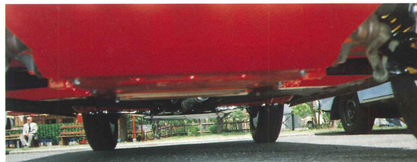
Fig. 5 The exhaust tucked up tight against the chassis.
