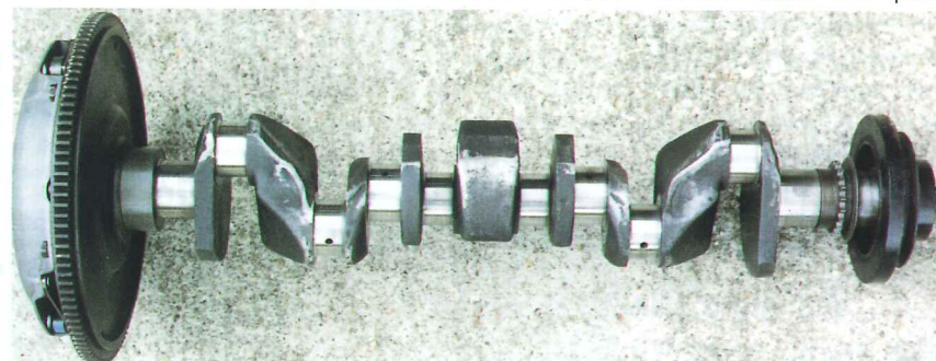
Fig. 4 The rotating mass balanced. Note the areas where frazing was removed
