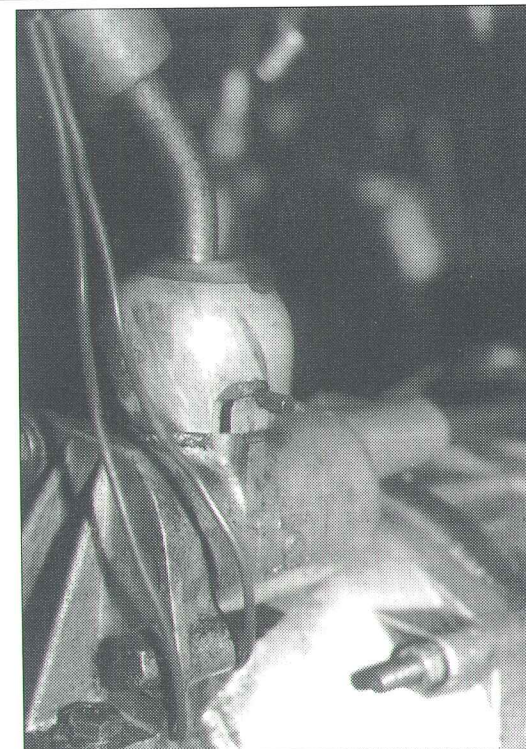
Fig 2. One of the gearstick locating pins had worked out allowing the gearstick to rotate
