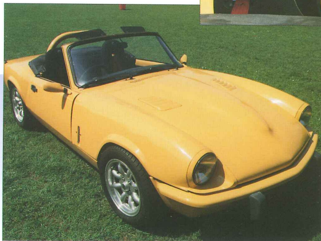
Paul Day's Spit with a GT6 bonnet. Re-moulded front and rear, with distinctive high brake light on the roll bar. Features in Triumph World Soon.
