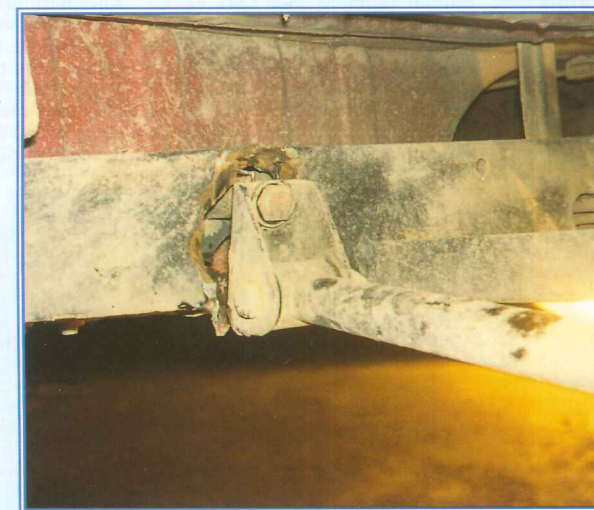
Rear radius arm pulled out of the N/S outrigger
