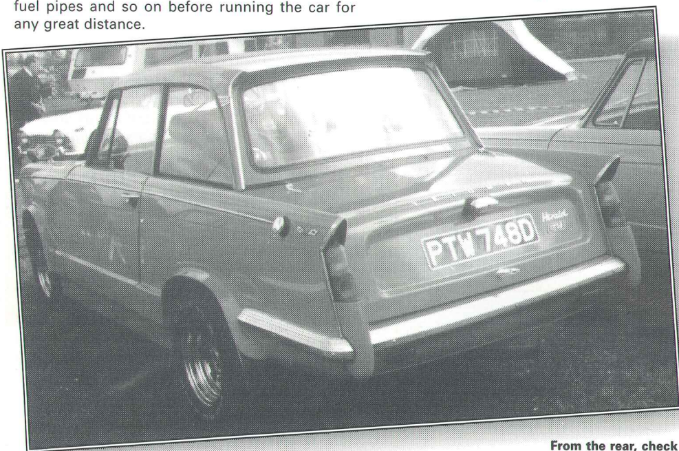
From the rear, check out the built in fog lamps and wheelarch extensions
