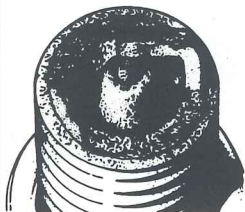
Excessive black deposits caused by over-rich mixture or wrong heat value
