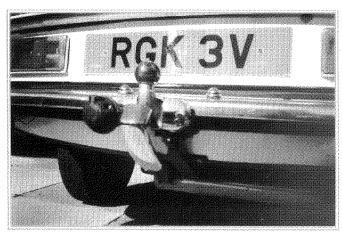
bolts securely to the underbody or chassis or the car. Our cars all have a strong chassis which is really the best and safest fixing point. Imagine the problems in fixing towing equipment to a Mini with its subframes. Aren't we lucky?
