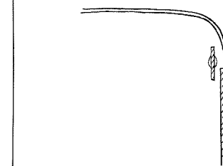
Fig. 4. Tucking the door glass under the hood. N.B. If the side of the hood is too long then this can't be done.
