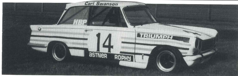
The other TRANS AM Vitesse (the Candy Box). The rear axle was replaced by KSC for a LSD type instead of welded up type.
