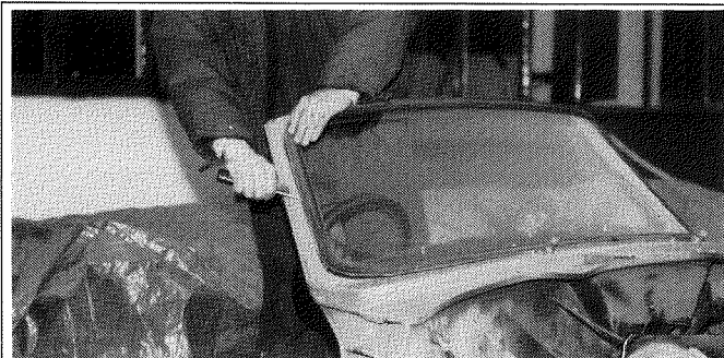
Fig. 4. Screen removal. This can be awkward, but the best method I have found is to run a blunt screwdriver around the outer seal to break the sealant. Repeat this inside the car, then apply a steady pressure on the inside of the glass, in the corners and at either side. I concentrate on the top edges, but try to keep things equal on each side.
