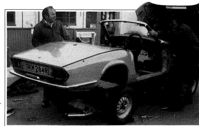
Fig. 14. As can be seen, you can then rest the tub on the rear wheels. Remember to chock them, to stop the chassis rolling out. Resting the tub on the wheels gives your team a breather too. Lift the front to level the tub, then with two people, lifting at the rear arches and two at the front corners. Lift and walk the tub back away from the chassis.
