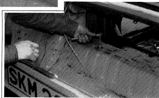
Fig. 12. . . . . using a long reach socket, remove the last pair of bolts. The body tub is now unbolted from the chassis. Go round each corner of the car and lift. This breaks the seal to the chassis and if it won't lift, you've missed something.
