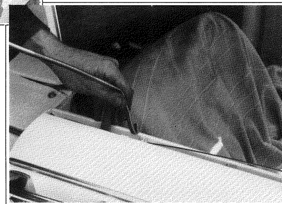
Figure 518. Make up a hook tool similar to that shown here (I made mine out of a flattened length of copper fuel pipe - but a length of stiffer metal would be better) and fix both the inner and outer door top seals in place.
