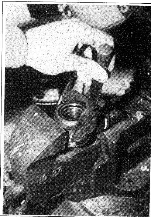
Figure 402. Unclip the clutch release mechanism from the bellhousing and separate off the clutch release bearing carrier. Support the bearing on top of the open jaws of a vice and knock off the carrier.
