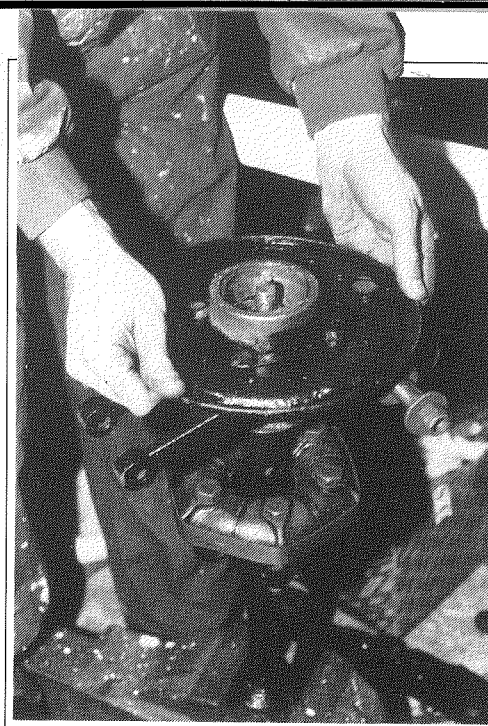
Figure 340. With the drive shaft supported in a vice, drop over the vertical link.
