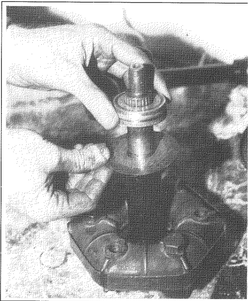
Figure 333. Double check that the facing plate hasn't been bent during its removal - if so flatten it straight and then place over the shaft followed by the inner hub. Note the elastoplasted thumb. Every home mechanic should have one!
