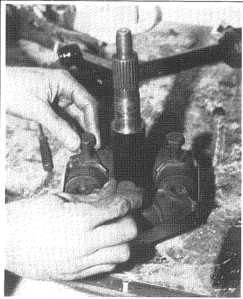
Figure 331. The relevant three of the six new coupling bolts can then be fed in. Spanner tight is OK at this stage.
