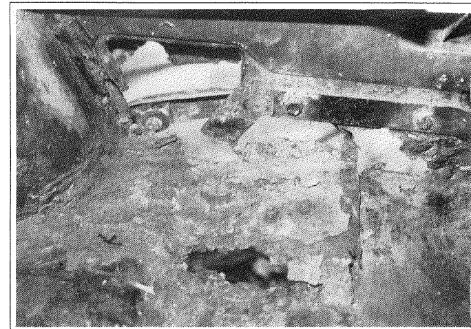
Figure 9. Extensive corrosion to the boot floor and the inner and outer rear wings!
