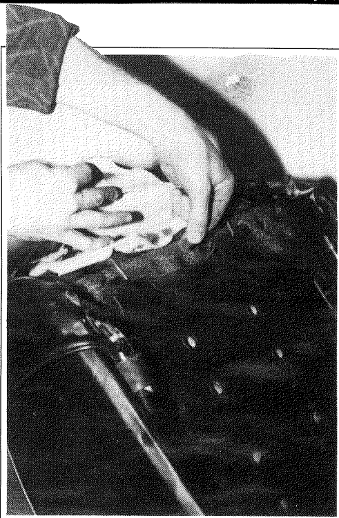
Figure 3. With the first rear flap pulled out of the way, a white calico flap can then be seen. This is the clever bit of the squab - to be revealed later and is attached to the rear frame with a single centrally placed clip. Prise this off. Ease the calico out of the frame and then remove the final single clip which secures the seat base cover to the rear of the frame.
