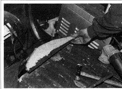
Figure 239. A repair was duly made up out of a solid section of one of the old rear wings previously removed. Recycling gets everywhere. Perhaps I thought that like a skin graft, the repair would be less likely to be rejected by the car sometime in the future if the replacement steel came from the same body!
