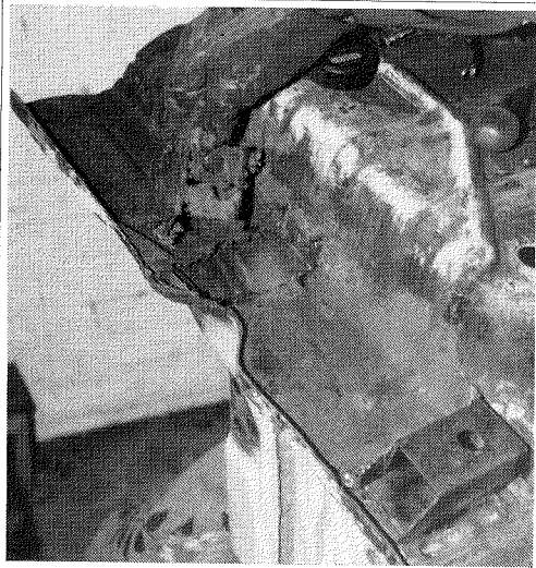
Figure 221. Continue the exercise to the rear of the bulkhead floor, removing all the rot...
