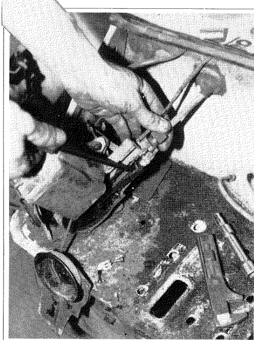
Figure 208. Back to the front, removing the windscreen wiper motor entails unscrewing the drive cable securing nut, then about 4 small screws, lifting off the top plate and then sliding off the top clip and electrical wiper. The drive crank pin can be prised out of its locating hole as shown here.
