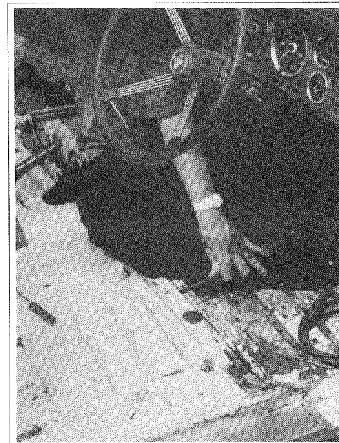
Figure 145. Unscrew the large self tapping bolts holding the front and rear sections to the centre outriggers and start to loosen off the joint which will be stuck together with old sealing goo.
