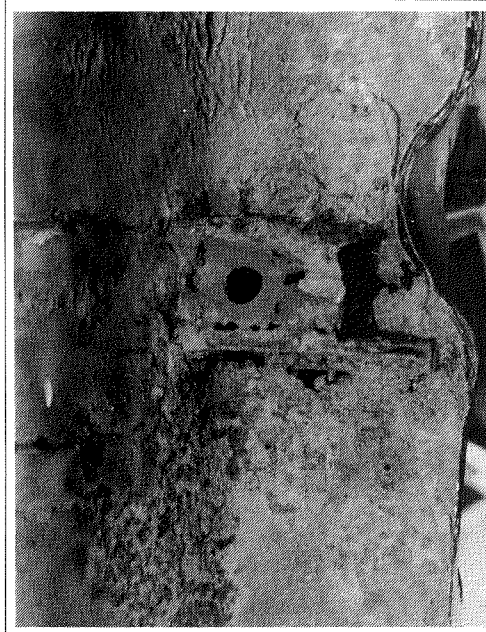
Figure 161. Just how did the car stay in one piece with front body mounting brackets like this? There's a bit of one of the driver's side still attached to the chassis as easily seen in figure 160!
