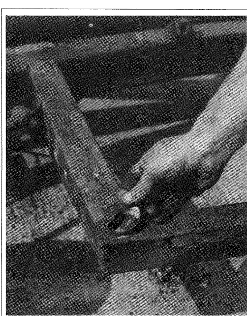
Figure 151. ...and a number of steel, slotted packing washers on the chassis side rails (the exact number will vary depending on the number used when the car was first put together).
