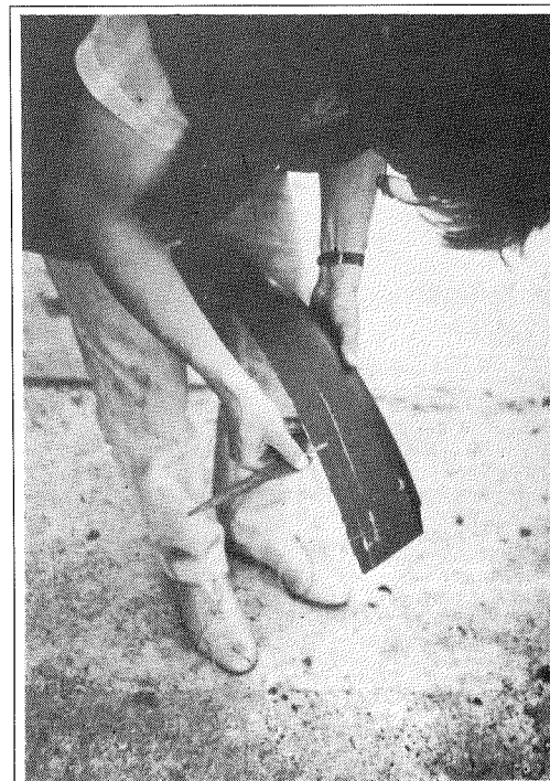
Figure 125. With the old wheel arch cut out, clip the repro panel around the wing lip (obviously if you're also replacing the rear wing and not yet welded that in place, you'll have to clamp the wing onto the car at the same time). Next, mark the inner edge of the panel where it meets the inner flange. Ensure that the wing is hanging properly at the same time as it tends to bow out slightly unless forced into place. From this scribe mark make another parallel line about half an inch outside of this to allow for making a return flange.
