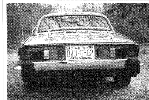
Figure 12. The large chrome bumper centre section and rear overriders fitted to Spitfire 1500s after 1975.
