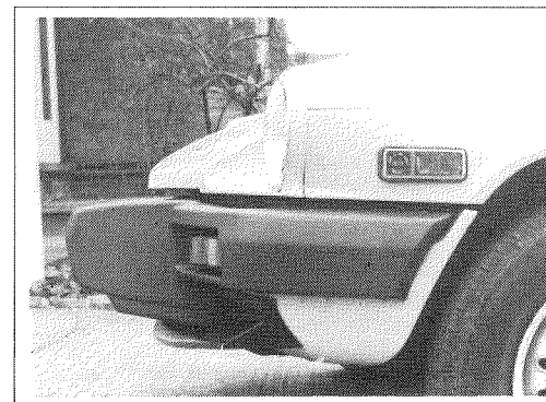
Figure 11. The more angular front spoiler and air cowl fitted to later US Spitfire 1500s.
