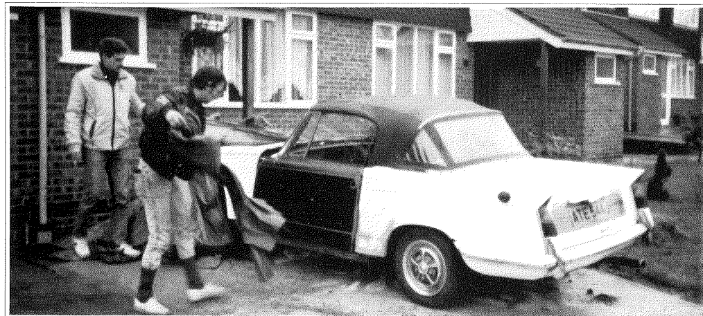
Figure 1. After over a year on the drive the car looked a little sad to say the least. Both rear wings were to come off and be replaced with fiercely sought after original panels together with one of the wing tops. Both rear outer wheel arches were also replaced: one with an original panel found via a Courier 'Wanted' ad, and the other with a repro panel. Fitting both will be covered in detail. If possible, always try for original panels as you know they should fit. There are some out there, you've just got to find them. As can be seen,
