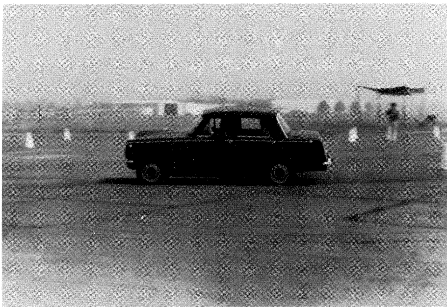
Practice Day — Gazel cornering at speed on fully deflated Denovo tyre. Photo: J. T. Yeomans.
